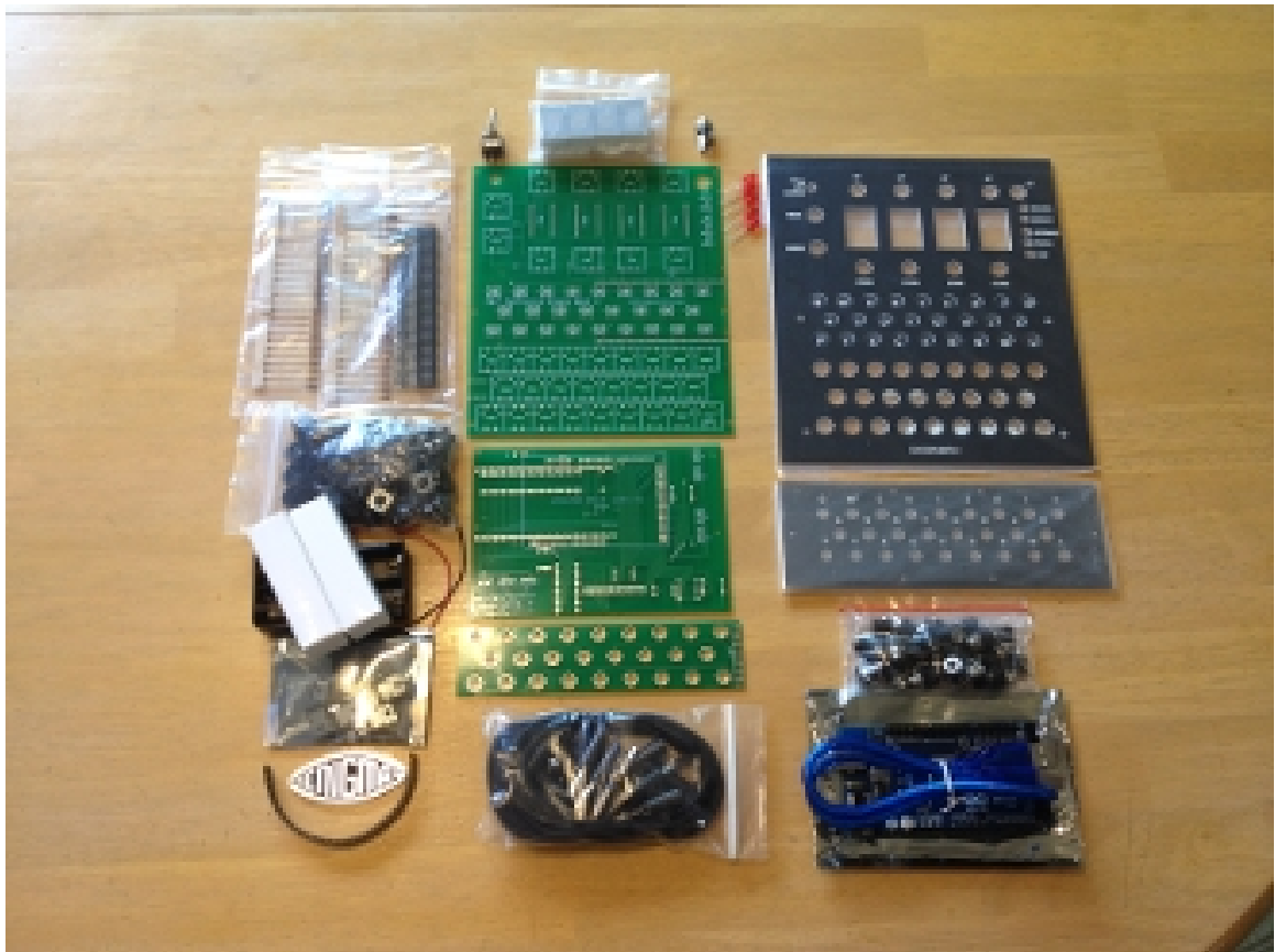
Figure 21: Mark 4 Enigma kit, pre-assembly; image taken by the author
