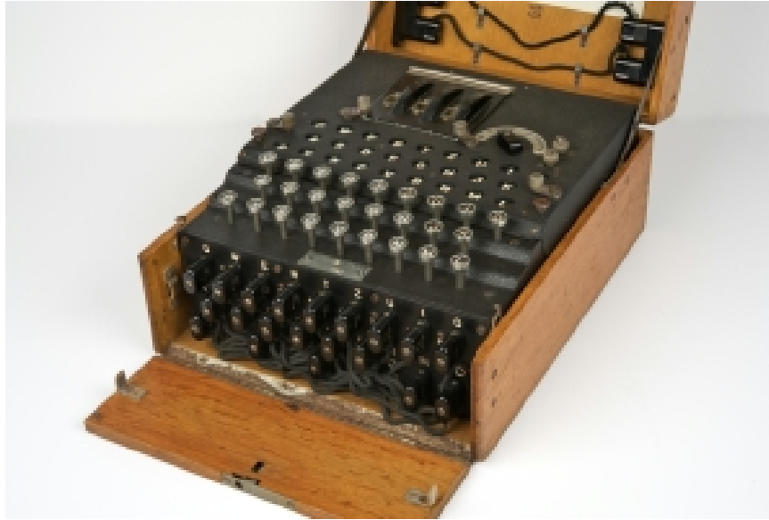
Figure 12: Enigma I ; image reproduced with permission of Crypto Museum [7]
