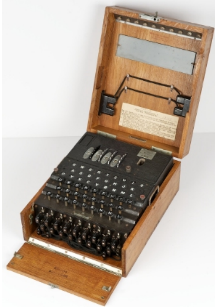
Figure 13: Enigma M4; image reproduced with permission of Crypto Museum [7]
